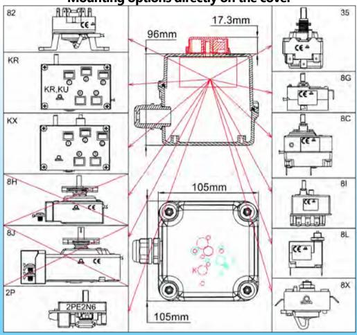
**Drilling references:** Replace the characters TT in the basic reference by the 2 characters located in the selected thermostat cell. **Attention:** the thermostat and eventually the knob and bezel must be ordered separately, see catalogue N°1.
